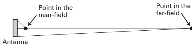
Figure 9.7 Fundamental geometries for antenna near and far fields.
