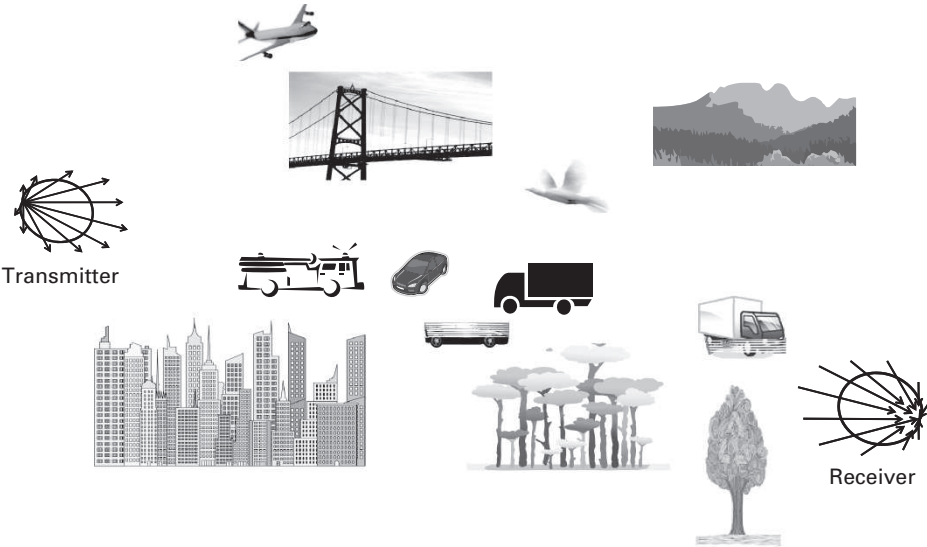
Figure 9.12 There are many, many possibilities for reflections of propagating EM waves on the way from a transmitter to a receiver.
